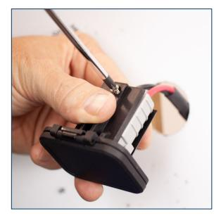
**NOTE** When the screws are tightened correctly, the mount will compress around the plug housing as shown here to eliminate sideways movement.
